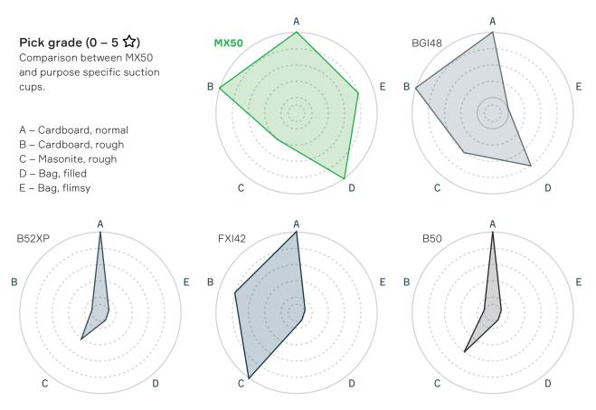
Testing performed using low vacuum flow with COAX® MICRO Si cartridges.
